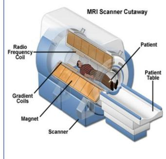
Another type of magnet found in every MRI system is called a **gradient magnet**. There are three gradient magnets inside the MRI machine, which are extremely low strength compared to the main magnetic field. The main magnet immerses the patient in a stable and very intense magnetic field, and the gradient magnets create a variable field.
